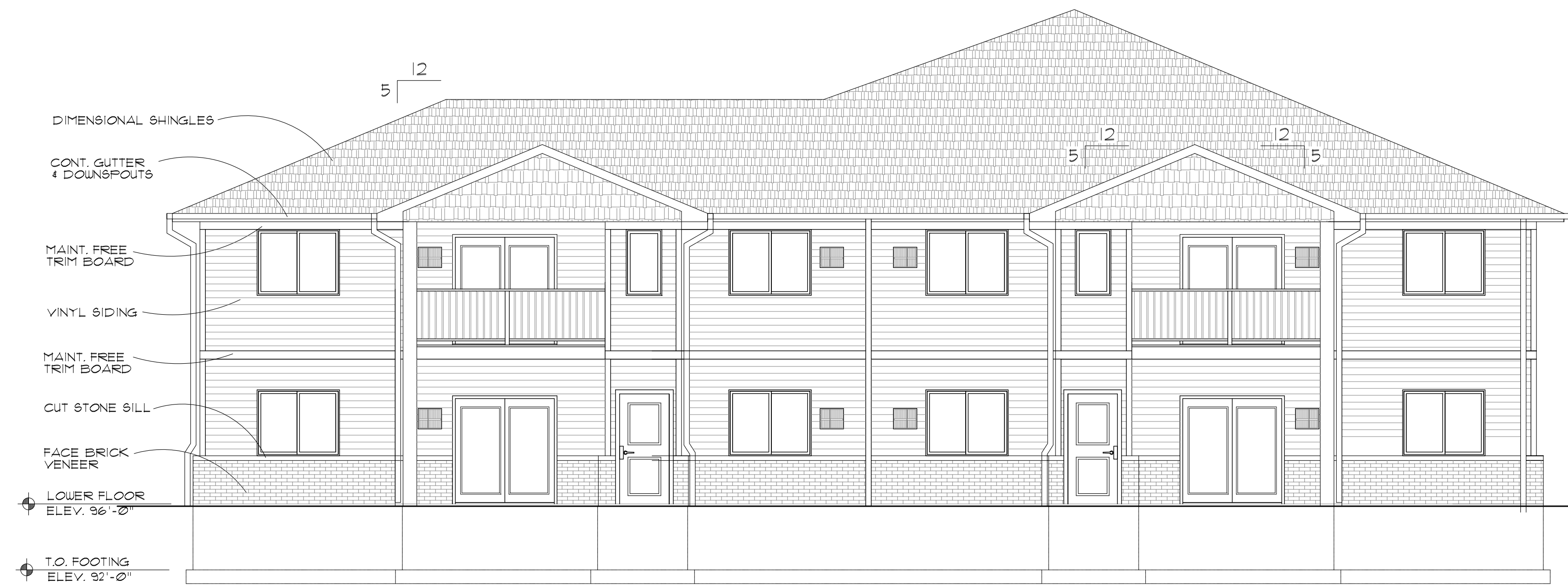
LOWER FLOOR SIDE ELEVATION SCALE: 3/16" = 1'-0"
