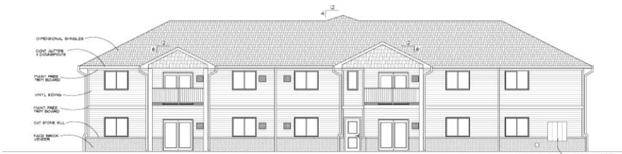
SIDE ELEVATION SCALE: 3/16" = 1'-0" OPPOSITE SIDE HATCHED SHADE
